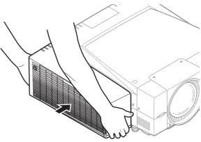
5 Hold the Smoke Resistant Box with one hand and use a Phillips-head screwdriver to tighten the four fixed screws to fix the box in place.
